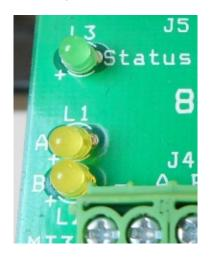
There are three LEDs on the backside of the unit.
