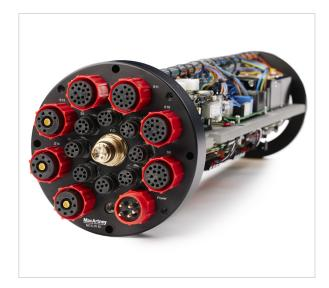
The MacArtney NEXUS 8 is a multiplexer capable of multibeam sonar, gigabit ethernet, HD video, and, additional sensors that are carried over one single-mode optical fibre via CWDM (Coarse Wavelength Division Multiplexing).
