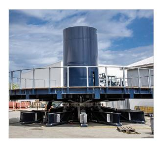
MacArtney CEMAC electrically driven carousel solutions are robust and energy-efficient cable handling systems that safely store and install on- and offshore power and telecom cables.
