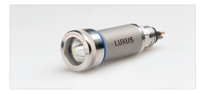
The LUXUS compact LED light is ideal for diving applications. The LED has an output of 440 or 780 lumen and is available with different reflectors. The LUXUS compact LED is a wet and dry light and can be used from 4,000 metres depth up to the deck without needing to be switched off. The electronics have an auto resetting thermal protection switch that protects the LED and LED driver from high temperatures.
