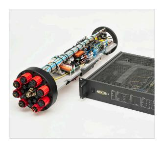
The MacArtney NEXUS 8 is a multiplexer capable of multibeam sonar, gigabit ethernet, HD video, and, additional sensors that are carried over one single-mode optical fibre via CWDM (Coarse Wavelength Division Multiplexing).
