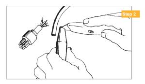
2. Cut pigtail wires on OM connector to approx. 2 cm from the brass body. Trim back tapered cable entry on boot until the cable is a snug fit (approx. 0.5 mm less than cable diameter).
