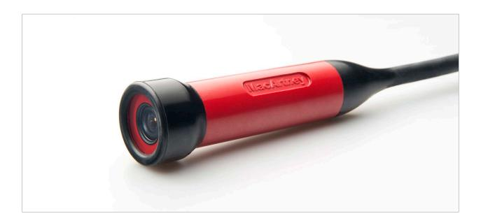
The LUXUS compact PUR (polyurethane) camera is a low-cost colour camera which is ideal for underwater operations. This light sensitive camera has a fixed focal length which can be factory adjusted to capture images at very close range. It can be equipped with different lenses for various angles of view.
