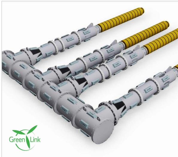
MacArtney HV GreenLink hubs are heavy-duty, dry-mate modular 'subsea sockets' made up to house multiple cables. Each module is mechanically linked to other modules using GreenLink inline termination technology. Extra sections can be added at initial launch or at a later stage, making the GreenLink hub a flexible option over time.
