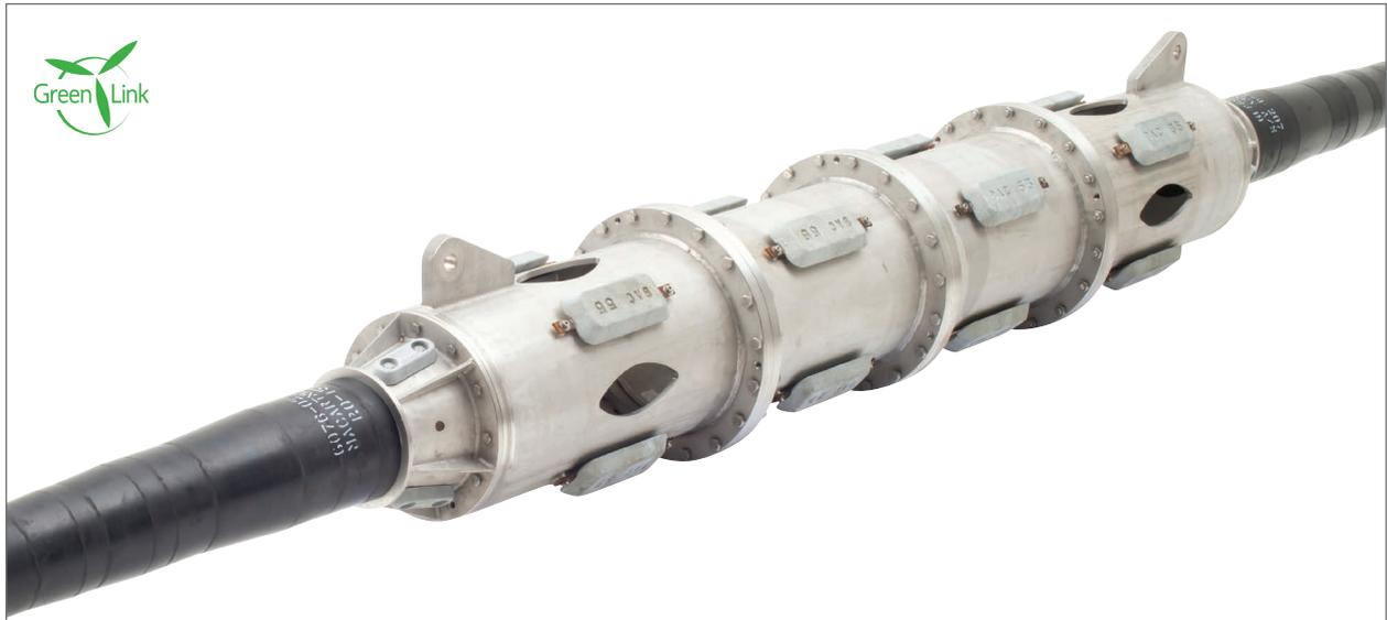
MacArtney GreenLink inline terminations have been designed to make offshore medium voltage termination jobs faster, easier and more efficient, hereby saving valuable ship time. These dry-mate systems are often used to connect dynamic cables from offshore renewable wind, tidal and wave energy converters to export cables. Moreover, they are widely used to interconnect subsea units.
