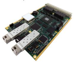
The Model 922-MES is a managed Ethernet switch implemented in a fully reconfigurable FPGA-based platform including DDR3 memory and two microcontrollers to support many existing and future protocols, as well as application specific code. Eight copper Ethernet ports and two optical Ethernet ports support many redundancy modes, including RSTP and MRP. Additional physical media redundancy on the optical ports provides fast, automatic, and protocol independent failover.
