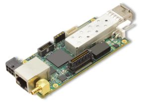
The Focal 914-HDE is an extremely compact, single card solution for High Definition (HD) video, Gigabit Ethernet and multiple serial data channels.
