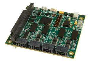
The 907-SER card is an 8-Channel RS-232/485 serial data expansion card intended for stacking on top of a 907 motherboard to add channel capacity. By default, this card is switch configured to multiplex eight data channels onto a single backplane data port (8:1) connected to a 907 motherboard. This default configuration has a maximum baud rate of 250 kbaud on each of the eight serial channels. Options include support for RS-422 configurations and higher data rates.
