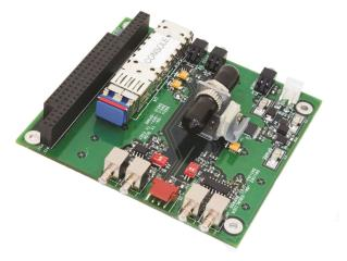
The 907-ECL (Emitter Coupled Logic) media converter provides optical transmission of high speed data formats typically used by sonars over a singlemode or multimode fiber. This card may be switch configured to support single-ended and differential ECL/PECL signals.
