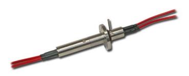
The Model 292 is an ultra-compact, two pass, multimode fiber optic rotary joint (FORJ). It is passive and bidirectional, and allows the transfer of optical signals on two separate optical fibers across rotational interfaces.
