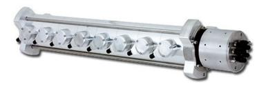
The Model 190 is a multipass fiber optic rotary joint (FORJ) for 2 to 17 multimode fibers. It is passive and bidirectional and allows the transfer of data, video and other signals on separate fibers across rotational interfaces.
