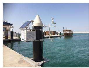
TideStation with VRS-20, Pressure and METPak with Solar Charging
