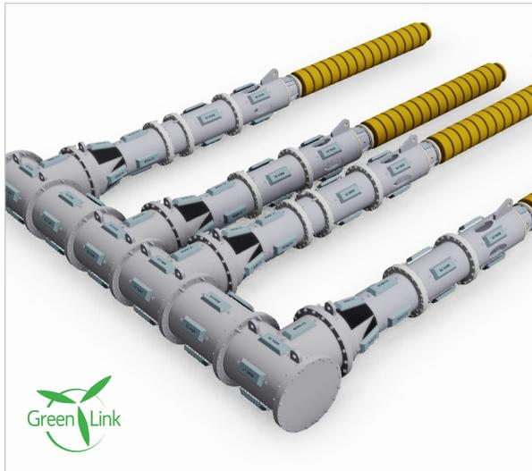
MacArtney GreenLink hubs are heavy-duty, dry-mate modular 'subsea sockets' made up to house multiple cables. Each module is mechanically linked to other modules using GreenLink inline termination technology. Extra sections can be added at initial launch or at a later stage, making the GreenLink hub a flexible option over time.
