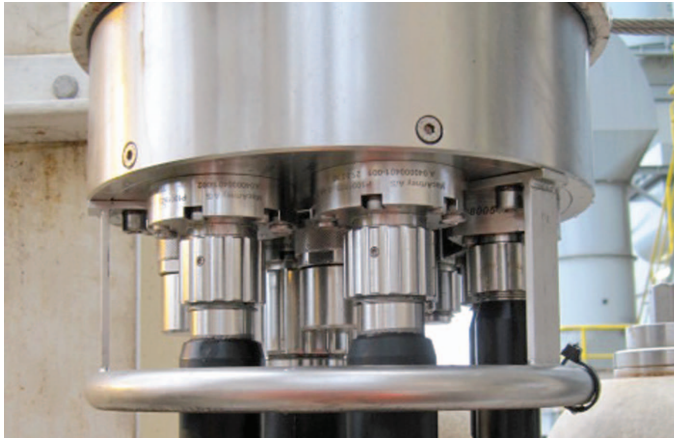
The connectors are also designed to be testable when mounted via two access points.
