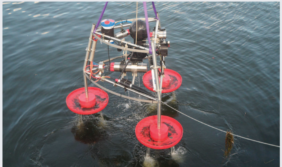
A complete MacArtney connectivity system is used to interface the multiple sensors onboard the UFO lander.
