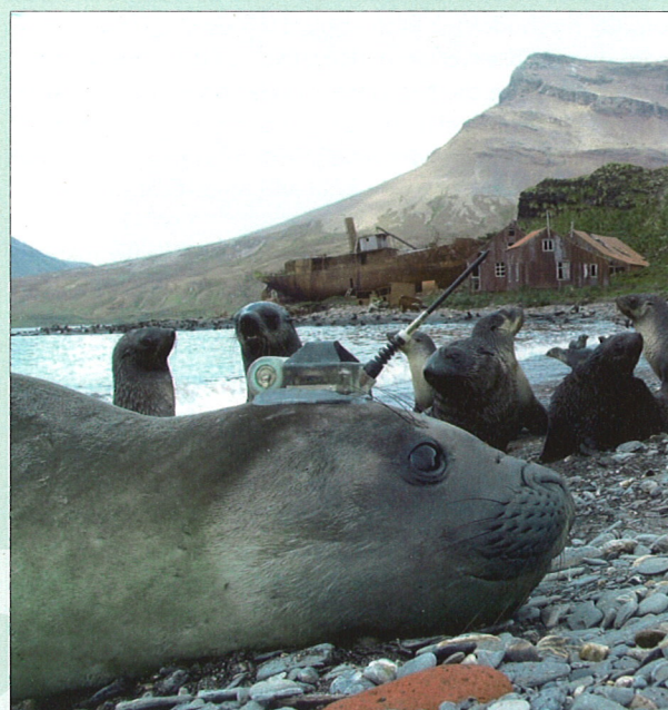
Female Elephant Seal wearing SMRU tag with Valeport CTD sensors.
