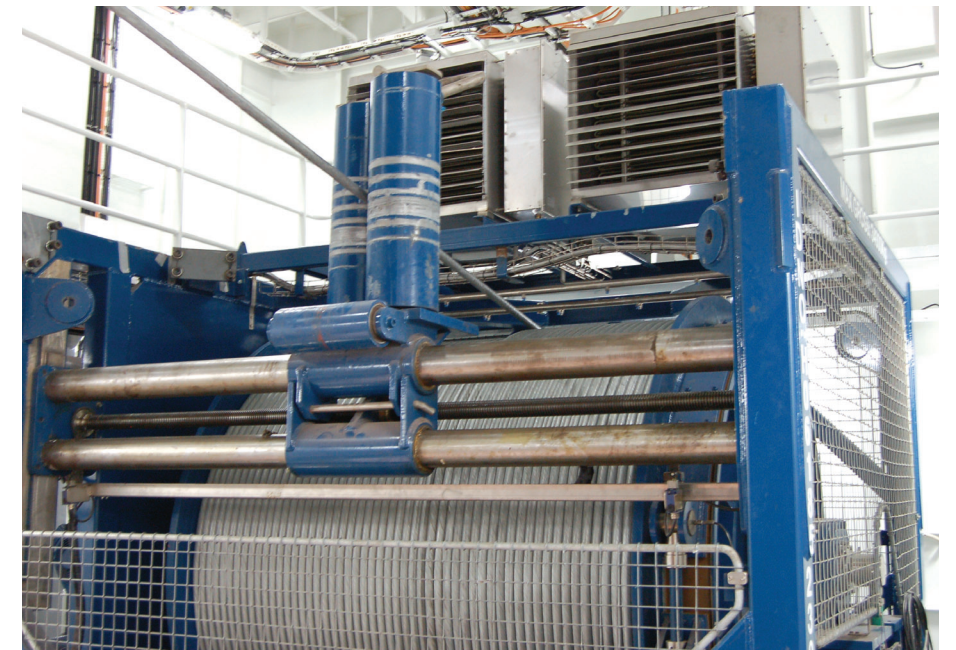
The PLC-controlled level wind
