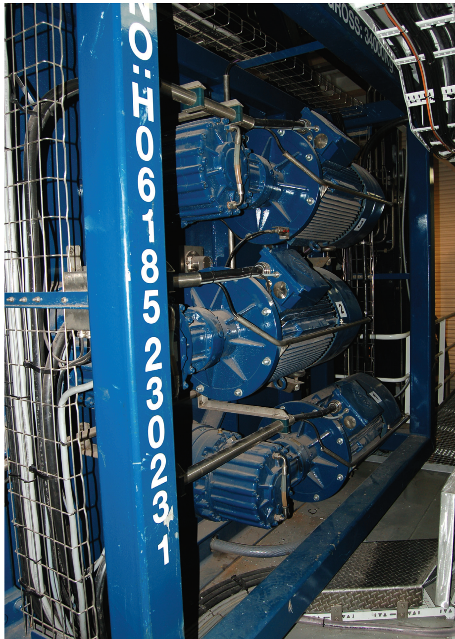
Three powerful electrical motors drive the AHC winch chosen by Oceaneering
