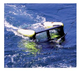
Adding a new dimension to towed vehicles, TRIAXUS is the natural step forward from the existing 2D towed vehicle technology to a true 3D towfish. TRIAXUS uses state-ofthe-art computer technology and fibre optic telemetry for vehicle and sensor communication.
