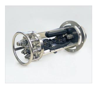
The TrustLink API FITA is a unique subsea connectivity system that assembles a harness cable or array of harness cables to a single cable, typically linking critical subsea control systems to an umbilical. Unlike other termination assemblies, the FITA can be assembled on site without the need for moulding.
