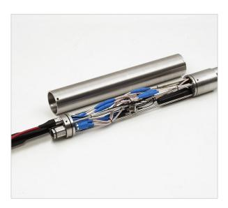
The TrustLink field installable termination assembly, or FITA, is a unique subsea connectivity system that assembles a harness cable or array of harness cables to a single cable, typically linking subsea control systems to an umbilical. Unlike other termination assemblies, the FITA can be assembled on site without the need for moulding.
