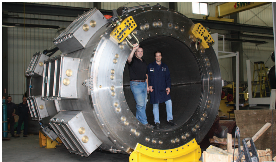
▲ Often comprising multiple electrical passes and fibre optical rotary joints Focal FPSO swivels can be rather sizeable systems
