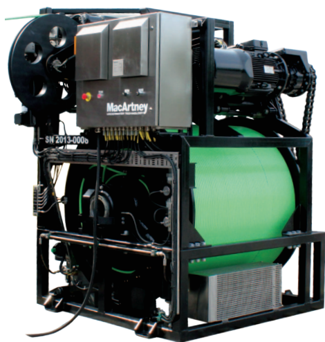
▲ The right angle MERMAC winch features Active Heave Compensation
