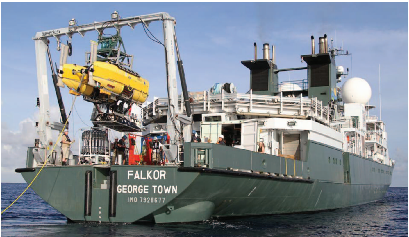
▲ The R/V Falkor uses its MacArtney Articulating A-Frame and a MacArtney ROV winch to launch and recover the WHOI HROV Nereus
