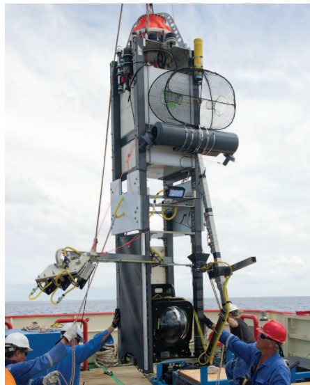
▲ SubConn® interfaced robotic landers descended to the abyss prior to the Deepsea Challenger
