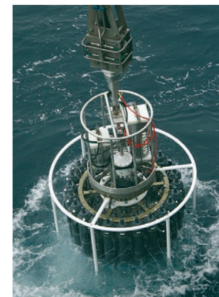
Profiling CTD systems and NEXUS telemetry systems were an important part of the Galathea expedition, sampling and testing water and assimilating valuable information on the oceans.
