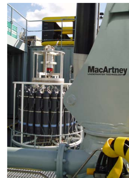
Profiling CTD systems and NEXUS telemetry systems were an important part of the Galathea expedition, sampling and testing water and assimilating valuable information on the oceans.
